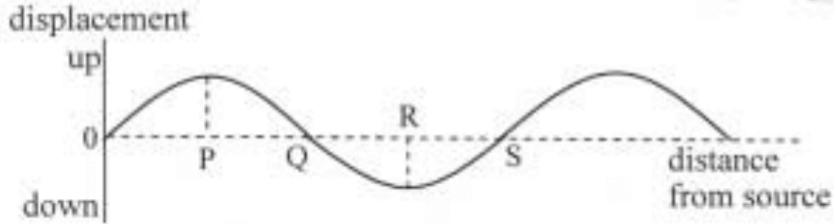
The graph shows, at a particular instant, the variation of the displacement of the particles in a transverse progressive water wave, of wavelength 4 cm, travelling from left to right. Which one of the following statements is **not** true?
