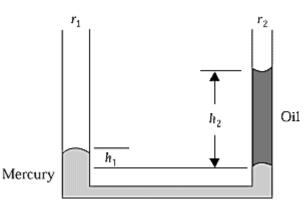
The left-hand side of an open U-tube has a radius  $r_1 = 0.82$  cm, and the right-hand side has a radius  $r_2 = 0.41$  cm. Mercury and oil are poured into the U-tube. The density of mercury is 13.6 g/cm<sup>3</sup>. The heights shown in the diagram are  $h_1 = 3.50$ cm and  $h_2 = 57.3$  cm. The density of the oil is approximately A) 0.83 g/cm<sup>3</sup> B) 110 g/cm<sup>3</sup> C) 7.9 g/cm<sup>3</sup> D) 6.9 g/cm<sup>3</sup> E) 1.82 g/cm<sup>3</sup>
