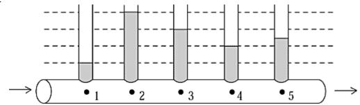
A pipe that appears to be of uniform size has constrictions on the inside. When a liquid flows through the pipe, the pressures at various points are indicated by the heights of the columns in the manometer tubes. If fluid friction is negligible, at which point is the diameter greatest?
