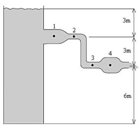
Water is discharged from the tank in the manner shown. At which point is the pressure the least?
