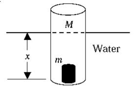
A cylindrical piece of wood has a mass M = 0.235 kg. A small piece of lead with a mass m = 0.021 kg is fixed in the wood at the bottom of the cylinder so that the cylinder floats in water in a stable position, as shown. The radius of the cylinder is 1.65 cm. The depth x of the cylinder below the surface of the water is
