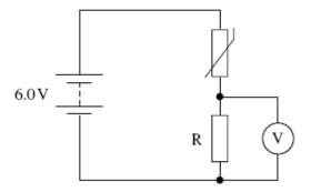
When the temperature is 50 °C the resistance of the thermistor is 1.2 k $\Omega$ . The voltmeter connected across *R* reads 1.6V.
