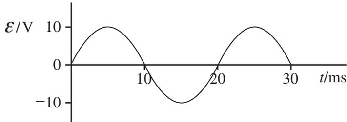
The above graph shows how the output emf,  $\mathcal{E}$ , varies with time,  $t$ , for a coil rotating at angular speed  $\omega$  in a uniform magnetic field of flux density  $B$ . Which one of the following graphs shows how  $\mathcal{E}$  varies with  $t$  when the same coil is rotated at angular speed  $2\omega$  in a uniform magnetic field of flux density  $0.5B$ ?
