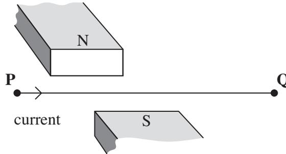
5 (a) (i) State the direction of the force on the wire when there is a direct current from **P** to **Q**, as shown in **Figure 5**.
