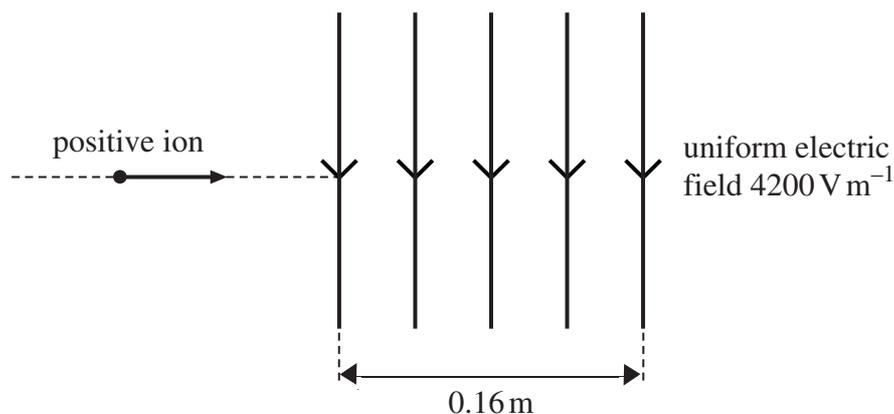
An ion carrying a charge of  $+4.8 \times 10^{-19}$  C travels horizontally at a speed of  $8.0 \times 10^5 \text{ m s}^{-1}$ . It enters a uniform vertical electric field of strength  $4200 \text{ V m}^{-1}$ , which is directed downwards and acts over a horizontal distance of  $0.16 \text{ m}$ .
