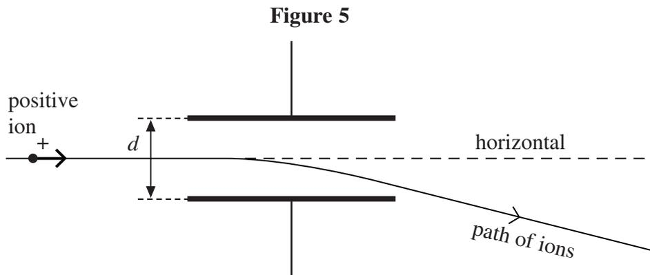
Whilst the electric field is still applied, the path of the ions may be restored to the horizontal, so that they have no overall deflection, by applying a magnetic field over the same region as the electric field. The magnetic field must be of suitable strength and has to be applied in a particular direction.
