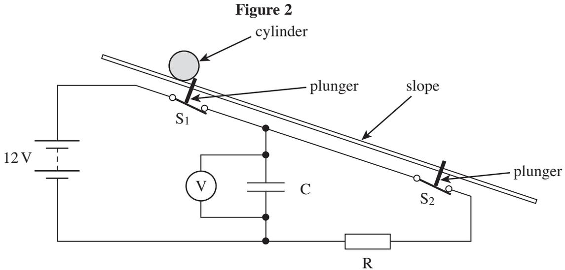
$S_1$  and  $S_2$  are two switches that would be opened in turn by plungers as the cylinder passed over them. Once opened, the switches would remain open. The cylinder would be released from rest as it opened  $S_1$ . The pd across the capacitor would be measured by the voltmeter.
