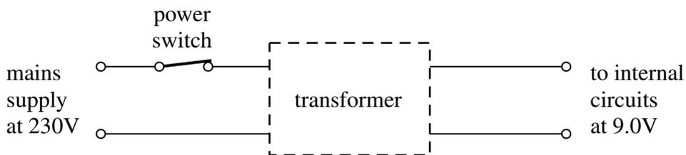
When in standby mode, the transformer supplies an output current of 300 mA at 9.0 V to the internal circuits of the TV set.
