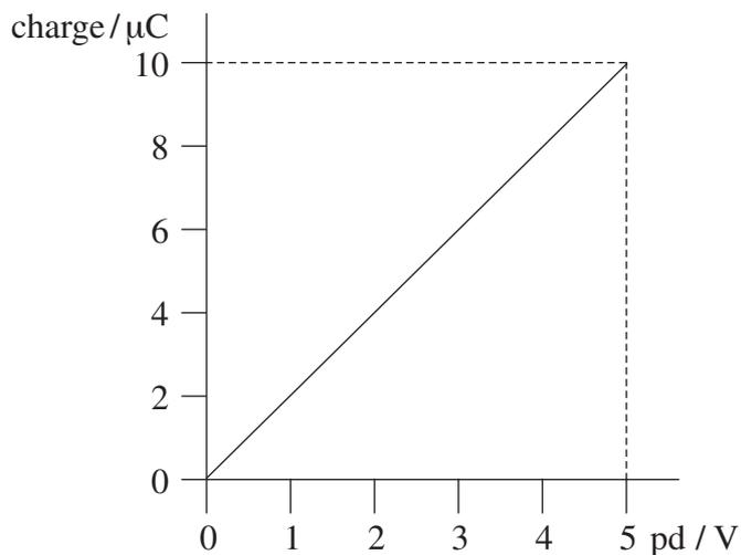
Which line, **A** to **D**, in the table gives the capacitance and the energy stored when the potential difference is 5.0 V?
